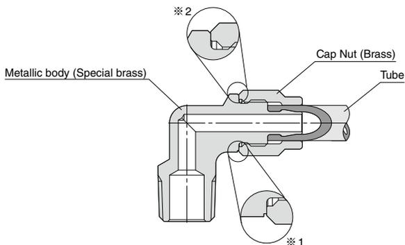
※ 1. Shape with Identification groove. Available tube I.D. :  $\varnothing 5$ ,  $\varnothing 6.5$ ,  $\varnothing 8$ ,  $\varnothing 11$ mm
